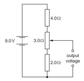
What are the maximum and the minimum output voltages of this potential divider circuit?
